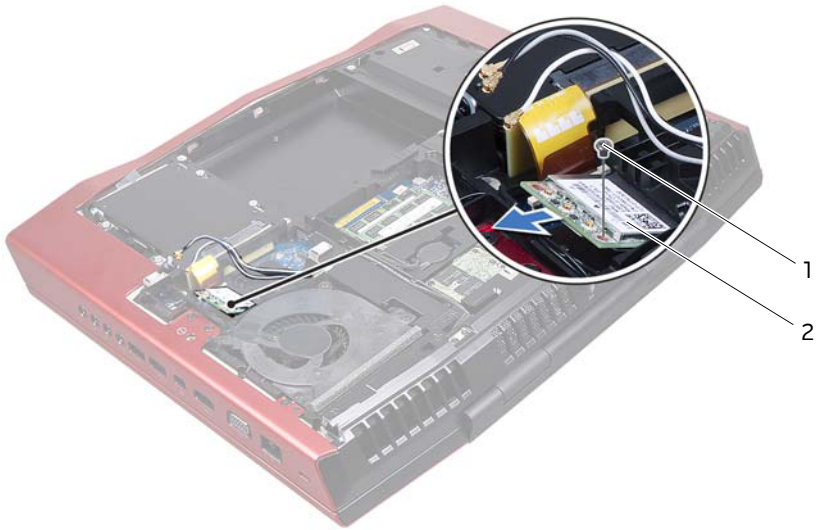
1 screw 2 wireless Mini-Card
